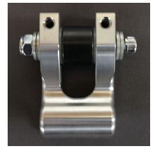
Replacing a 1  $\frac{1}{2}$ " roller bolt with a 1  $\frac{3}{4}$ " roller bolt and four washers will add 5.8 grams per arm.
