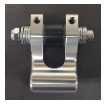
Replacing a 1  $\frac{1}{2}$ " roller bolt with a 2" roller bolt and eight washers will add 11.3 grams per arm.
