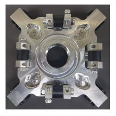
Allen screws must be added in pairs opposite to one another to keep the TAPP Clutch balanced. Adding two allen screws will add 5.2 grams.
