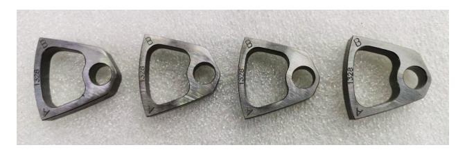
Flipping two opposing ramps from position "A" to "B" will increase RPM engagement and result in a harder shift profile. For drag racing, flip all four ramps to position "B". This will further increase engagement and result in an even more aggressive shift profile.
